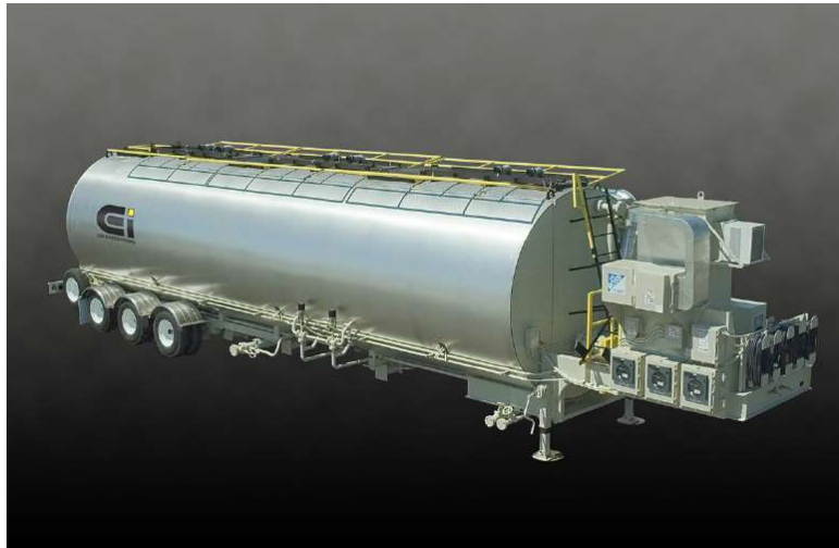
Figure 2-8. Example of asphalt rubber reaction tank (CEI Enterprises, 2008)
