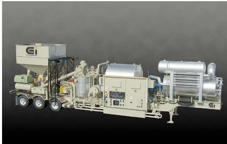
Figure 2-7. Example of on-site asphalt rubber blending plant (CEI Enterprises, 2008)
